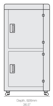
1544 x 926 x 2137mm External dimensions (WxDxH) 60.8 x 36.5 x 84.1" 635kg Weight Build volume 695 x 385 x 1200mm dimensions (WxDxH) 27.3 x 15.2 x 47.2" LCD screen 8K Resolution 7680 x 4320 pixels Print layer thickness 50-350µm Compatible with Daylight resins 3.3kW in average, 5.5kW Power consumption at peak Light output intensity 1.6 mW/cm<sup>2</sup> Light output 460nm wavelength Power input 32A 230v Single Phase Plug type 3 pin IEC60309 Warranty 12 months
