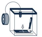
Place **P-surface 141** with the PPprint logo upwards on your printer bed and fix it with gentle pressure using the **P-roller 621**. You have also the option to adhere **P-surface 141** to your printer bed by using **P-adhesive 220**.
