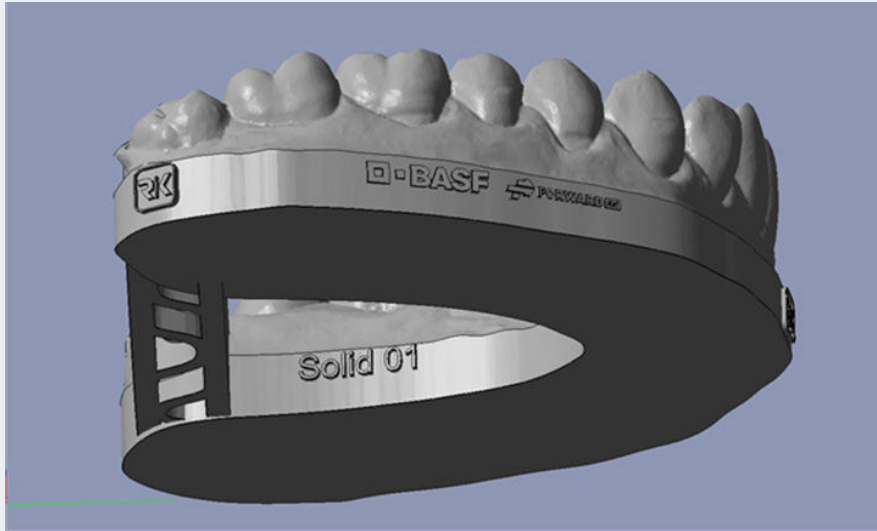
Figure 7: Solid created model with the exocad® Model Creator. (Source: Chitu Box Software, Organical CAD/CAM)
