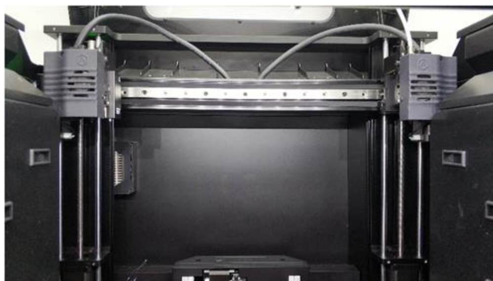
Figure 2 Lift the X axis to a proper height.
