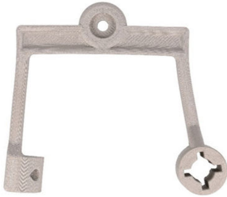
Figure 21. Part with distortions after D&S
