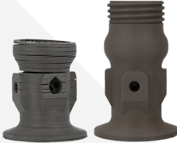
Figure 19. Cooling & Delamination example
