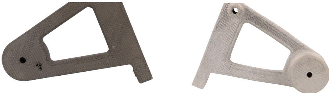
Figure 18. Damaged Bottom surface & resulting top cracks
