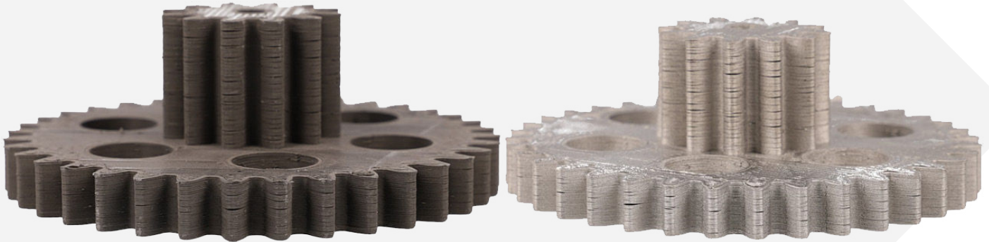
Figure 20. Print Delamination become sintered cracks
