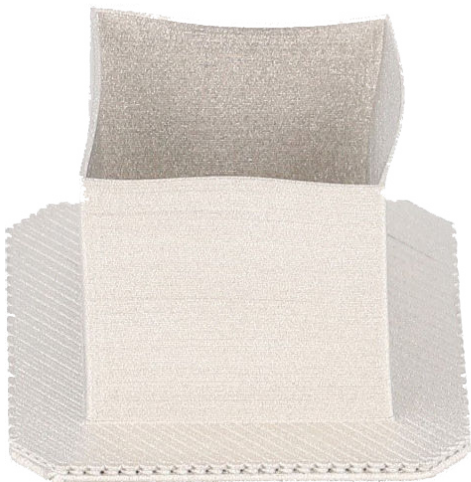
Figure 12. 0,4 mm Wall Failure
