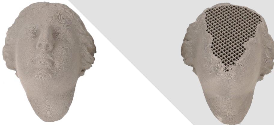
Figure 25. Mass reduction using infill
