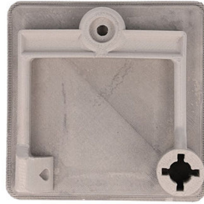
Figure 22. Use of shrinkage plate ensure uniform shrinkage
