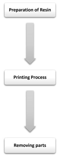
The material should be processed at room temperature. Before usage the material should be shaken well. Pour it slowly in the vat and wait a couple minutes, until smooth, bubble-free surface is obtained before starting the print job.
