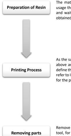
The material should be processed at room temperature. Before usage the material should be shaken well. Pour it slowly in the vat and wait a couple minutes, until smooth, bubble-free surface is obtained before starting the print job.
