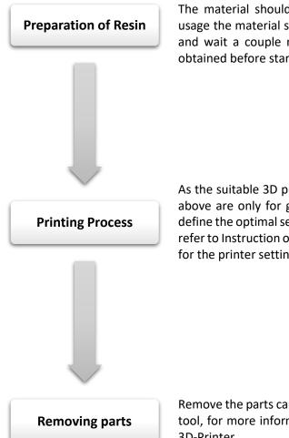
The material should be processed at room temperature. Before usage the material should be shaken well. Pour it slowly in the vat and wait a couple minutes, until smooth, bubble-free surface is obtained before starting the print job.
